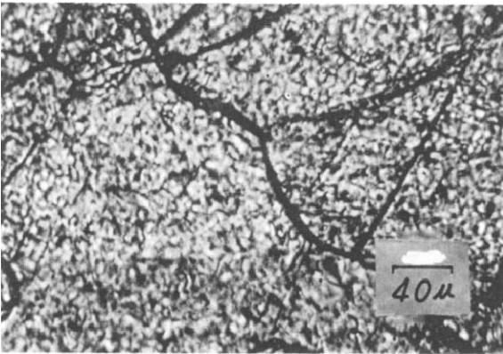
Fig. 3. Thin section showing appearance of typical marble and scattered mesoporosity (in black). Original magnification 200 \times .
